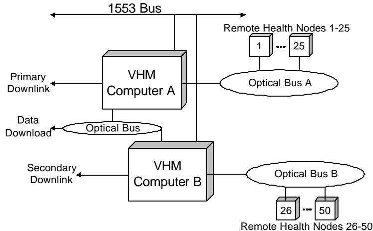
**Figure 1. Schematic diagram of Vehicle Health Management system**
