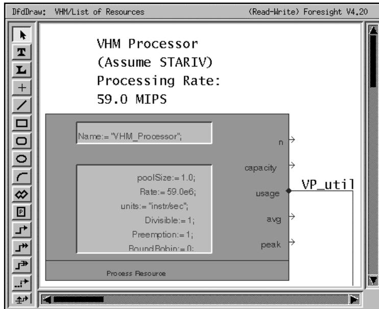
**Figure 6. Resource modeling of the VHM processor**
