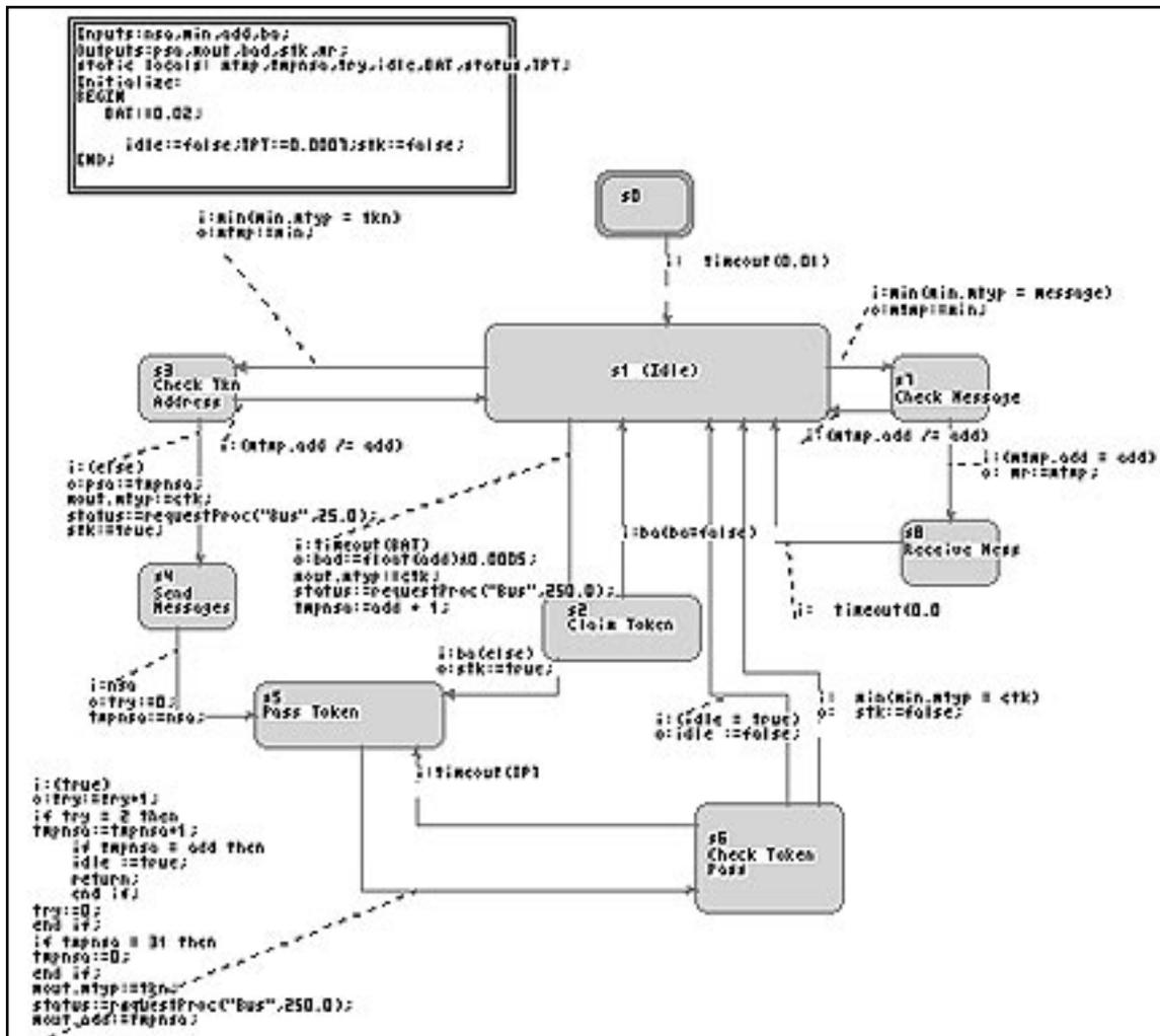
Figure 4. Foresight State Diagram Easily Captures Protocol Specifications
